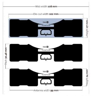
As we have our own antenna design capacity, we adapt to the most common chips in the RFID market, such as Impinj and NXP. At Trace ID, the verification process of each RFID tag is done through Voyantic, thus guaranteeing maximum performance.
