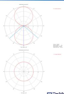
As we have our own antenna design capacity, we adapt to the most common chips in the RFID market, such as Impinj and NXP. At Trace ID, thanks to the use of Genesys software the verification process of each RFID tag is done through Voyantic, thus guaranteeing maximum performance.
